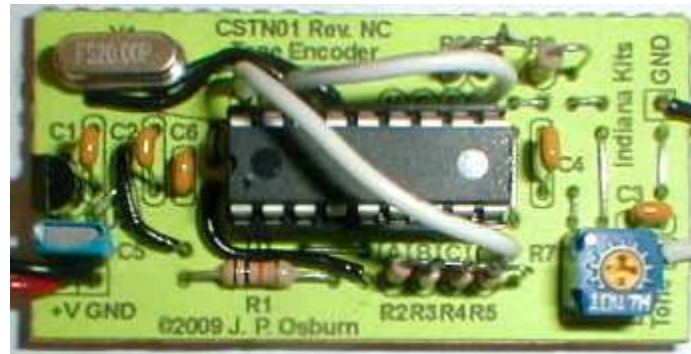
Figure 1 - CSRX01 Circuit Sticker Tone Encoder
